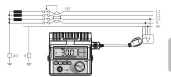
Single phase RCD test used in the TN system, like the following picture:
