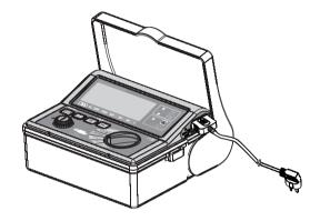
➤ Connect the test lead to the power supply socket. (The instrument is opened at this time, and the LCD begin to display).
