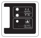
▶ If the green CORRECT WIRING LED not turn on, please disconnect the test lead when the red DO NOT PROCESS LED is light, and then check if the L and N lead also the ground lead is properly connected.
