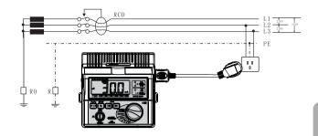
Connect the instrument to the system, and then check all the three lead, the CORRECT WIRE LED should light on.
