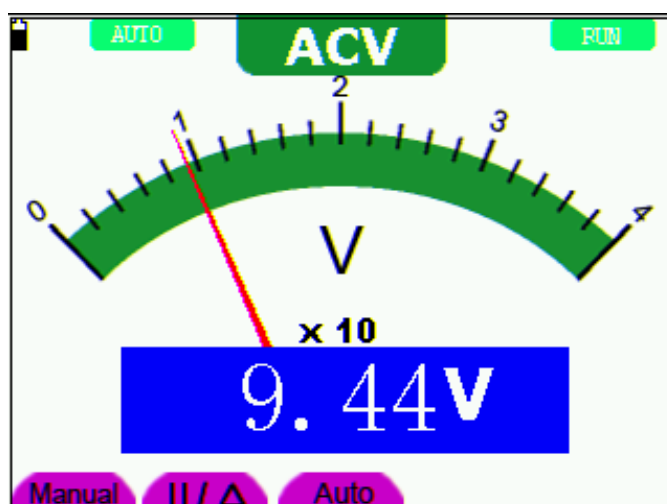
Figure 26: AC Voltage Measurement
