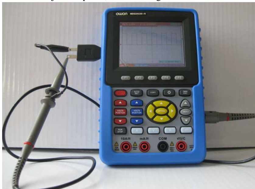
Fig.3. The connection of Square-wave test signal
