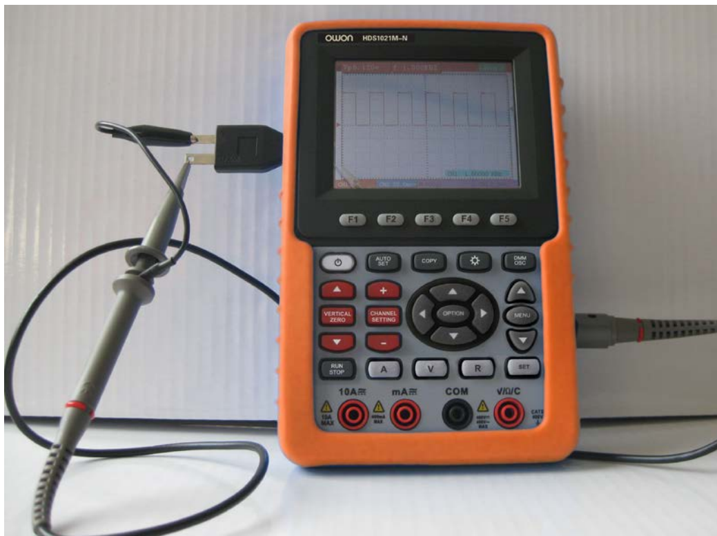
Fig.3. The connection of Square-wave test signal
