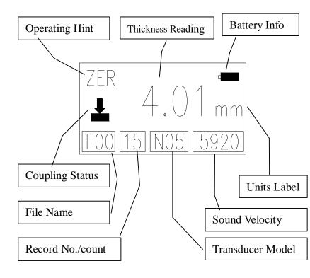
**Battery Information**: Display the information of the rest capacity of the battery.
