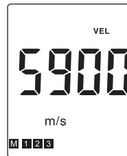
Last applied sound velocity & registered unit
